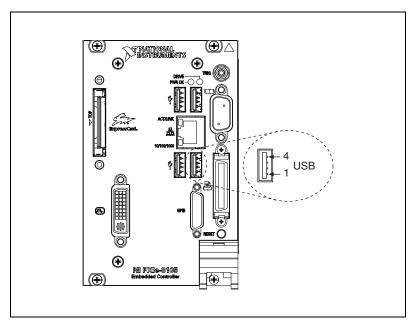
Figure 3-6. USB Connector Location and Pinout
